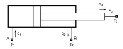
For example, the model of a double-acting hydraulic cylinder shown in the previous illustration can be described with a simple set of equations:
