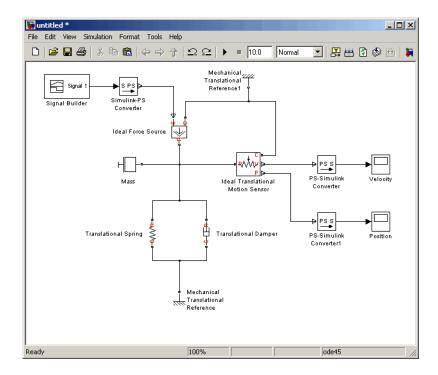
11 Each topologically distinct physical network in a diagram requires exactly one Solver Configuration block, found in the Simscape > Utilities library. Copy this block into your model and connect it to the circuit by creating a branching point and connecting it to the only port of the Solver Configuration block. Your diagram now should look like this.
