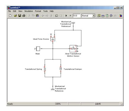
**9** Now you need to add the sources and scopes. They are found in the regular Simulink libraries. Open the Simulink > Sources library and copy the Signal Builder block into the model. Then open the Simulink > Sinks library and copy two Scope blocks. Rename one of the Scope blocks to Velocity and the other to Position.
