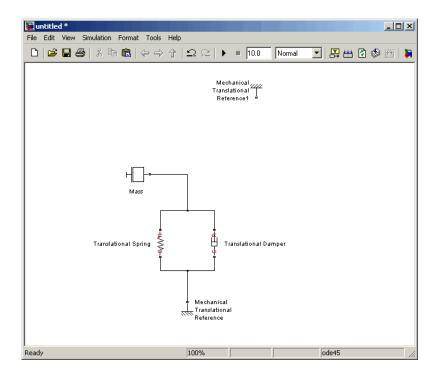
7 To add the representation of the force acting on the mass, open the Simscape > Foundation Library > Mechanical > Mechanical Sources library and add the Ideal Force Source block to your diagram.
