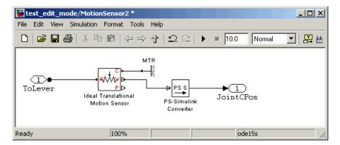
**4** Try to simulate the model. An error message appears saying that the model cannot be compiled because its topology has been changed while in Restricted mode. You can either undo the changes, or switch to Full mode, as described in "Switching from Restricted to Full Mode" on page 4-21.
