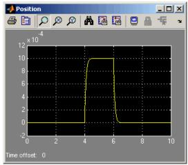
In the beginning, the mass is at rest. Then at 4 seconds, as the input signal changes abruptly, the mass velocity spikes in the positive direction and gradually returns to zero. The mass position at the same time changes more gradually, on account of inertia and damping, and stays at the new value as long as the force is acting upon it. At 6 seconds, when the input signal changes back to zero, the velocity gets a mirror spike, and the mass gradually returns to its initial position.
