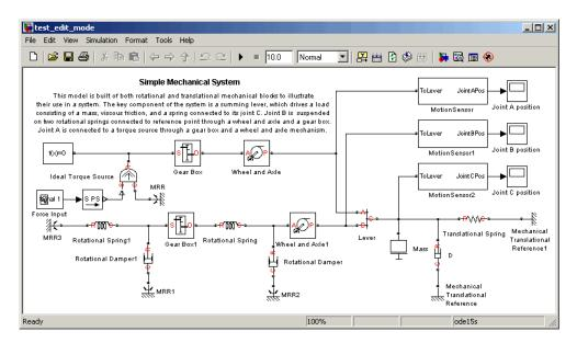
**2** Open the Joint C Position scope and simulate the model.
