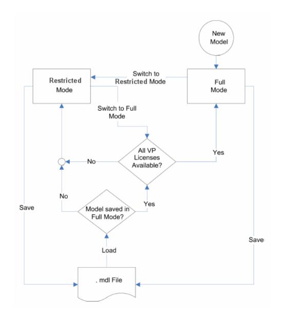
New models are always created in Full mode. You can then either save the model in Full mode, or switch to Restricted mode and save the model in Restricted mode.
